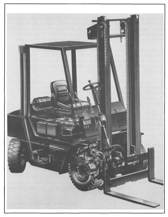
Modern hydrostatic drive forklift truck (Courtesy: Boss Trucks Ltd.)
